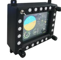
Highly reliable APM 5.6" cockpit display has been designed and built in SERBIA by TELEOPTIK -Gyroscopes Electro-Opto Mechanics military facility.
